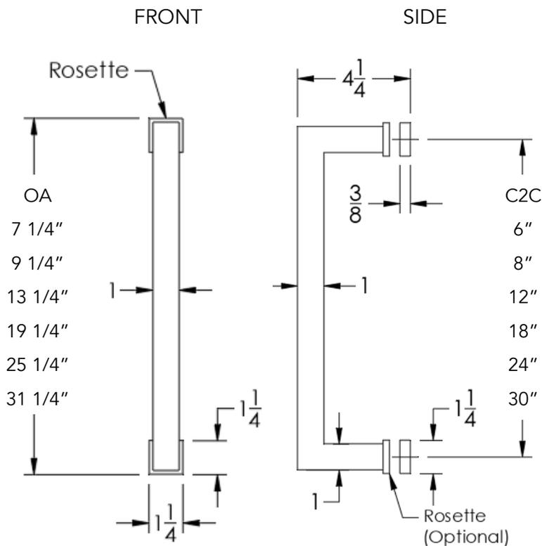
**Installation Notes:** Center to center hole drilling dimension are same as mentioned in column.
